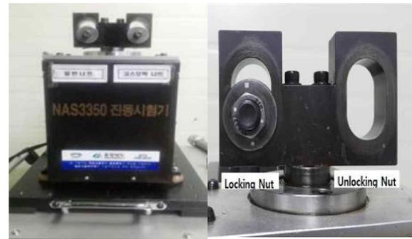
(a) NAS3350 tester (b) Nut with clamping jig
