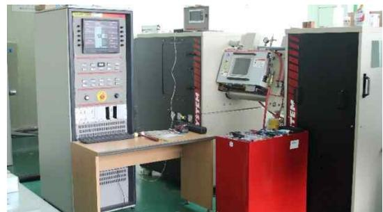
Fig. 1 Test equipment (Gleeble-3500)
