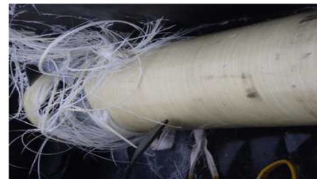
Fig. 6 Photograph of external defect (test 1)
