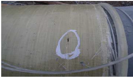
Fig. 8 Photograph of external defect (test 2)
