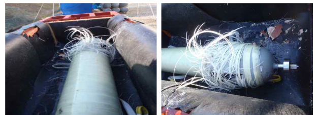
Fig. 4 Photograph of test result (after repeated pressure)
