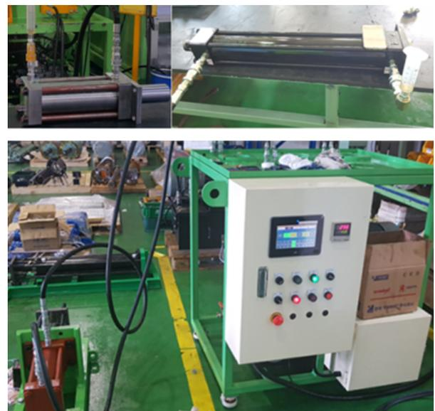
**Fig. 6 Performance test-bed of hydraulic cylinder**
