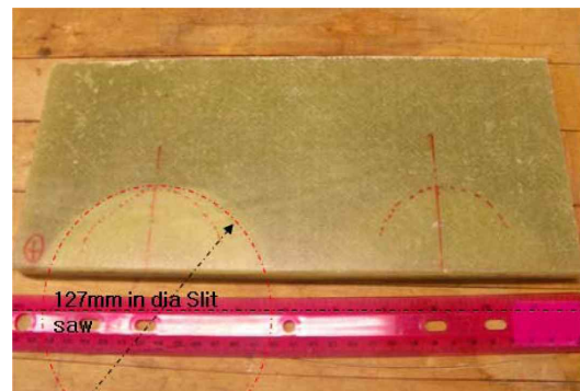
(a) GFRP composite laminate with saw cuts
