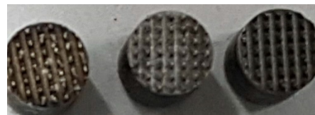
Fig. 2 Check patterned electrodes of which diameter is 4 mm. The number of each spike is 34
