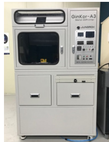
Fig. 9 Prototype of metal 3D printer
