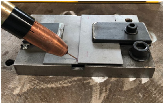
Fig. 2 Welding specimen and CMT welding jig used in the experiment
