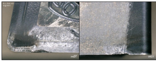
(a) Tool wear condition
