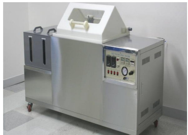
Fig. 8 Equipment of the Salt Spray Test
