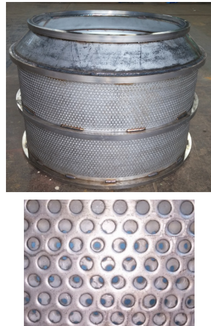
Fig. 4 A basket with several holes for agitation of plating solution
