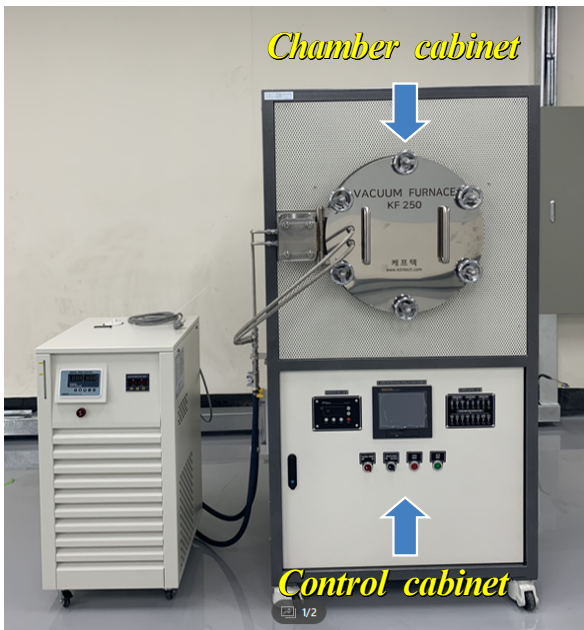
Fig. 4 Vacuum & Gas tight furnace KF-250
