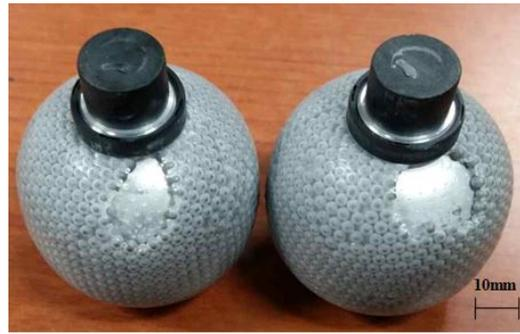
**Fig. 6 Defective products with incomplete injection molding**
