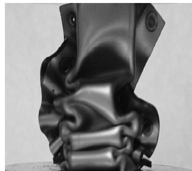
**Fig. 10 Shape of collapsed STD specimen**
