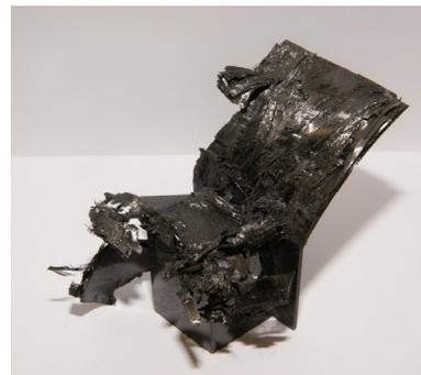
**Fig. 4 Shape of collapsed CFS specimen**
