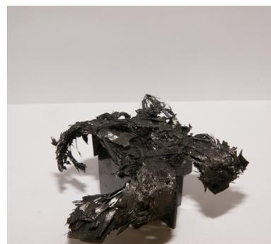
**Fig. 6 Shape of collapsed CFD specimen**
