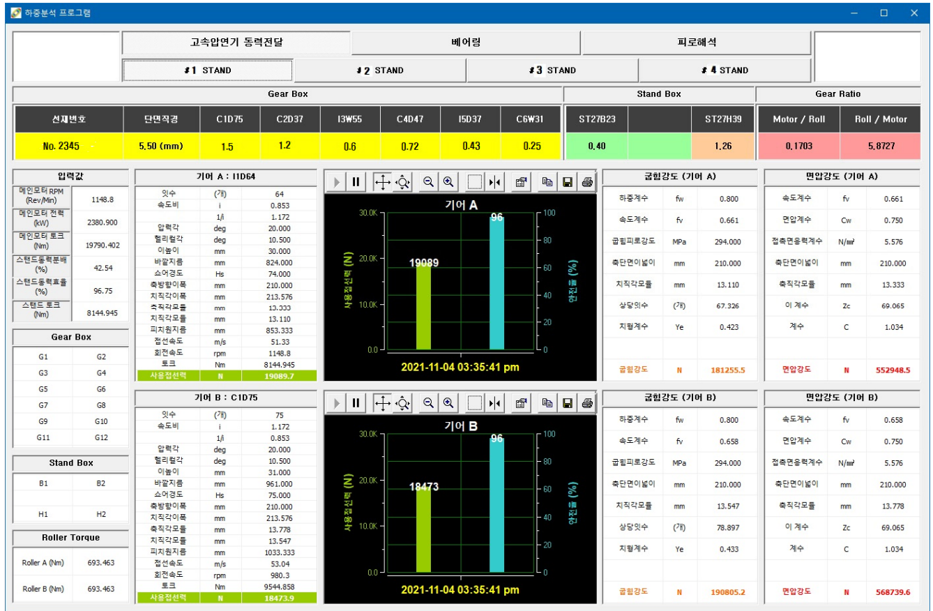
Fig. 12 Wire rolling system diagnosis and monitoring GUI
