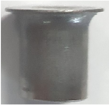
Fig. 16 Heading finished SPR
