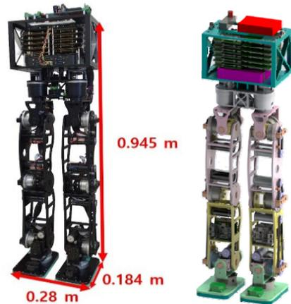
Fig. 2 Photograph and 3D model of SUBO-2
