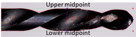
(b) Principle for measuring diameter
