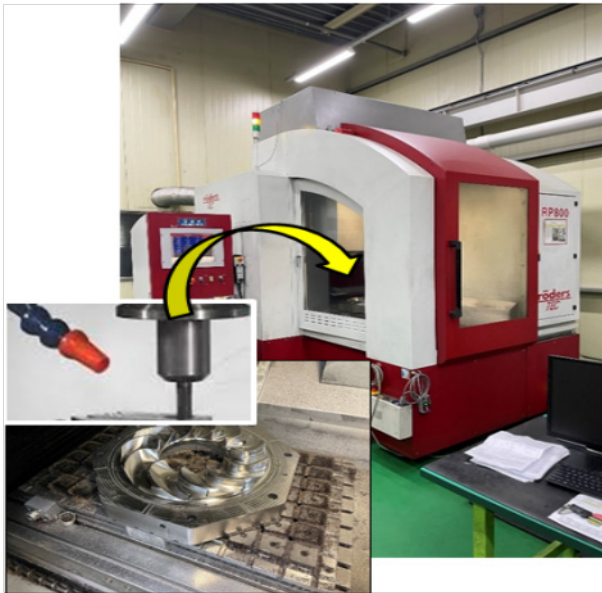
Fig. 5 RODERS_3axis CNC_milling machining center
