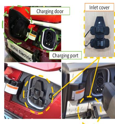
Fig. 2 Charging port parts of electric vehicle
