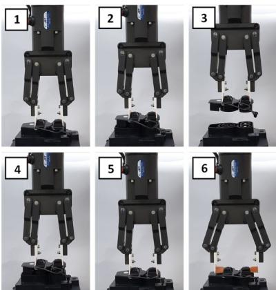
Fig. 11 Inlet cover gripping performance test using shape-adaptive soft gripper tip
