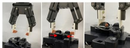
Fig. 5 Gripping inlet cover with shape-adaptive soft gripper tip
