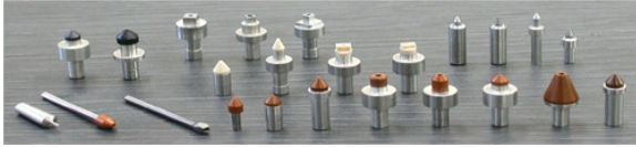
Fig. 2 Pick and place tools and various types of collets
