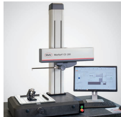
Fig. 11 Test equipment for burr height measurement
