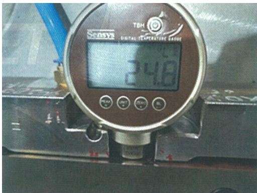
Fig. 10 Blanking temperature measurement of lower die of tail gate hinge
