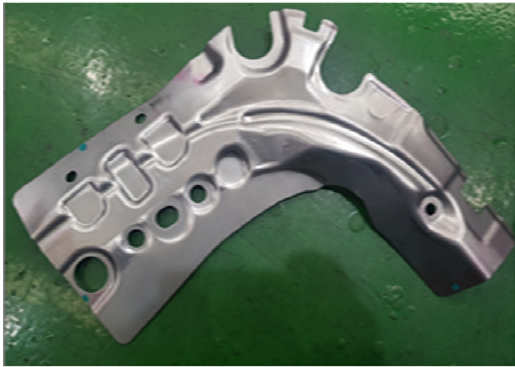
Fig. 13 Final product of tail gate hinge
