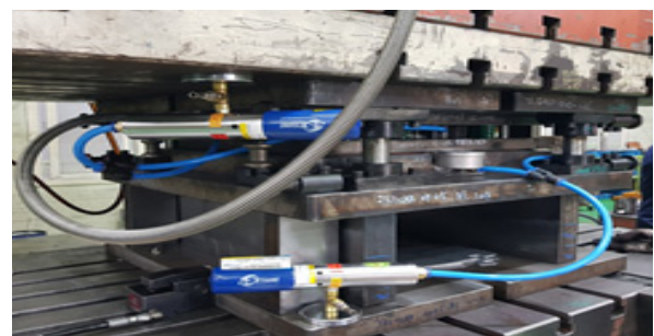
Fig. 8 Tail gate hinge die using rapid air cooling system with vortex tube
