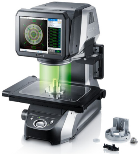
Fig. 3 Equipment for measurement – IM-7500
