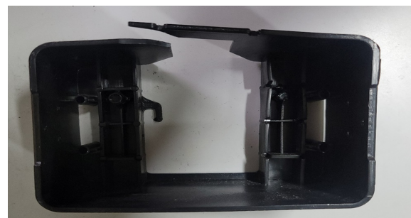
(b) Mole rat trap part - failure
