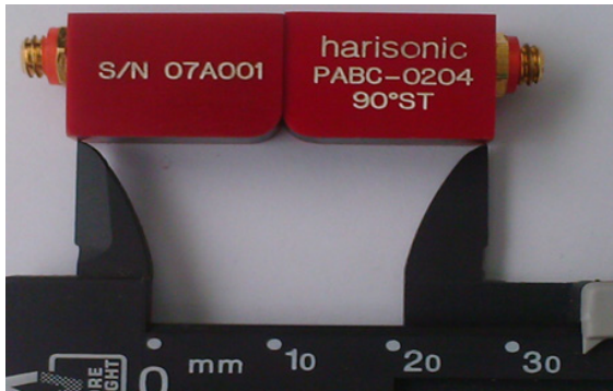
Fig. 2 Ultrasonic wave transducers for generating Rayleigh wave
