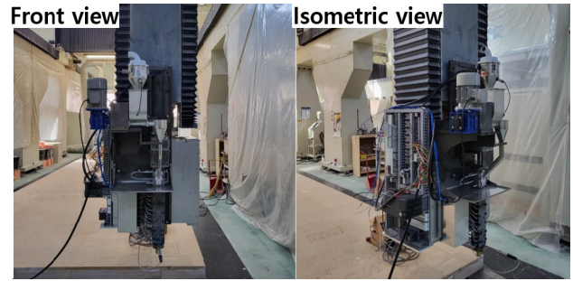
Fig. 3 Prototype of twin-screw extrusion additive manufacturing system
