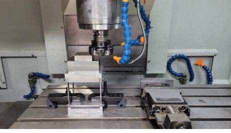
Fig. 16 Face milling process for the upper surface to ensure the surface flatness
