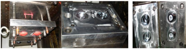
Fig. 5 Simultaneous injection mold for first and second apparatus of flexcage
