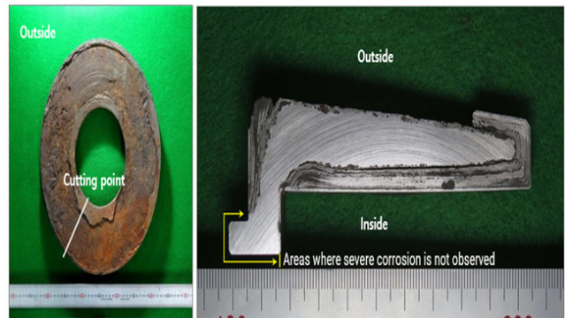
Fig. 4 Shape after cutting of the cross section of the damaged area
