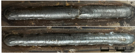
Fig. 11 Top bead appearance with worn machined contact tip
