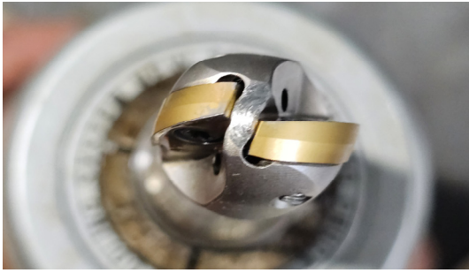
Fig. 4 Roughing ballendmill for stainless still
