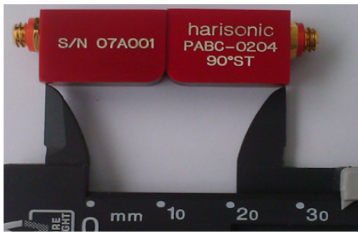
Fig. 2 Ultrasonic wave transducers for generating Rayleigh wave
