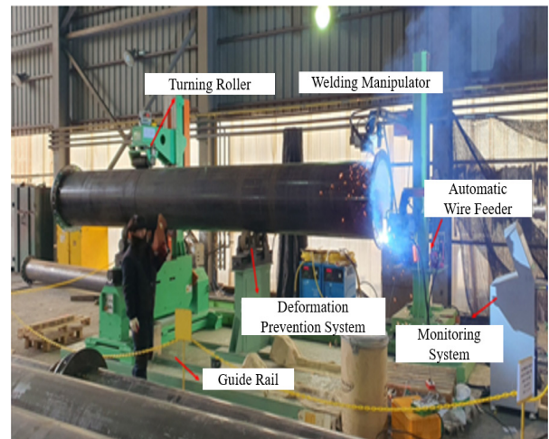
Fig. 6 Configuration of welding system in pipe-flange
