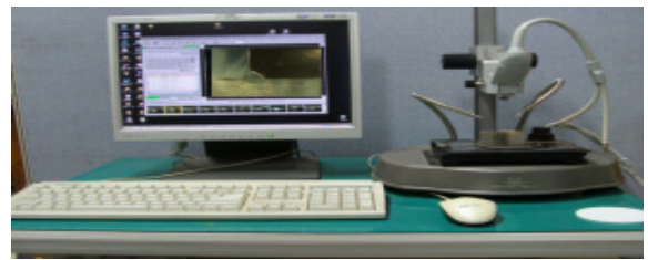
Fig. 4 Measurement of bead geometry
