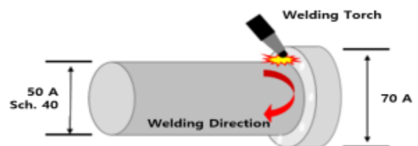
Fig. 1 A schematic diagram for GMA weld process
