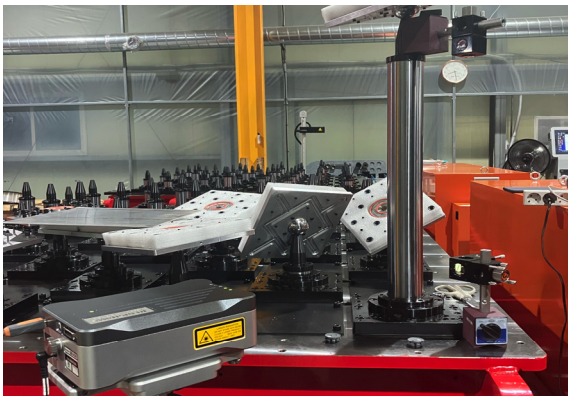
(b) Universal holding fixture
