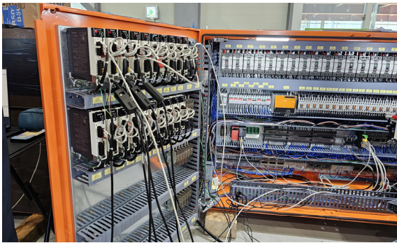
Fig. 2 Active fixing cylinder control system
