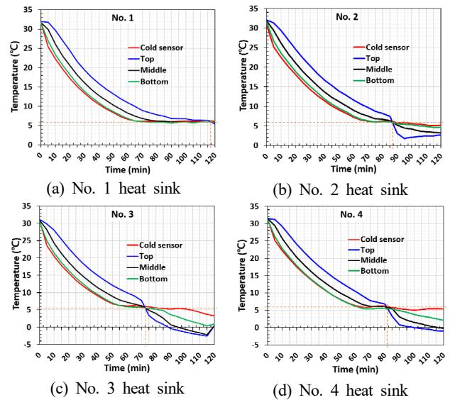
**Fig. 8 Temperature distribution of cold water and cold water tank by position according to heat sink**
