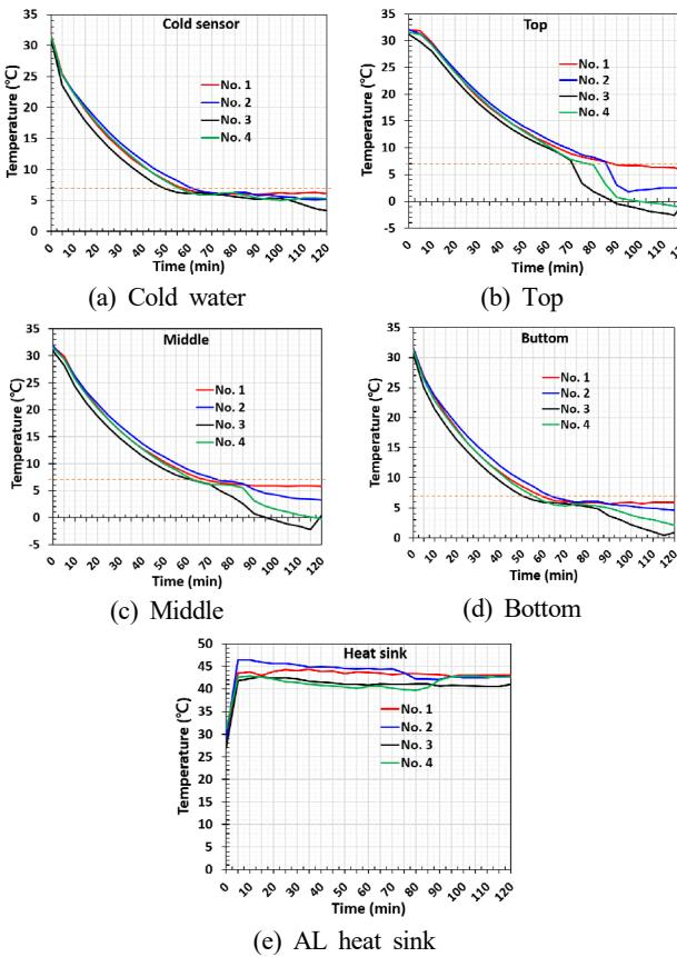
**Fig. 7 Comparison of temperature distribution at each position according to the installation of four types of heat sink**
