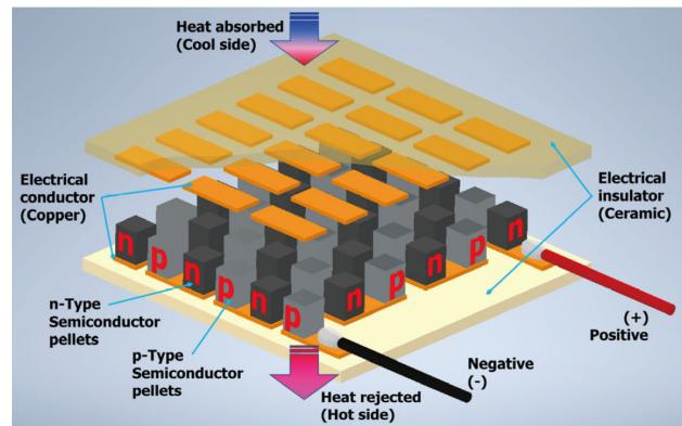
Fig. 1 Inner structure of thermoelectric element(TEM)
