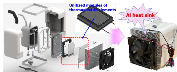
Fig. 2 Cold water tank with thermoelectric unit
