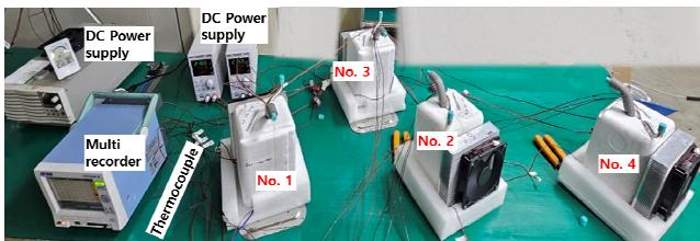
Fig. 5 Comparison of cooling performance of Z Co. TEM unit using AL heat sink
