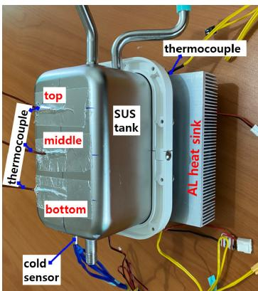
Fig. 6 Thermocouple installation location of cold water tank Assy'
