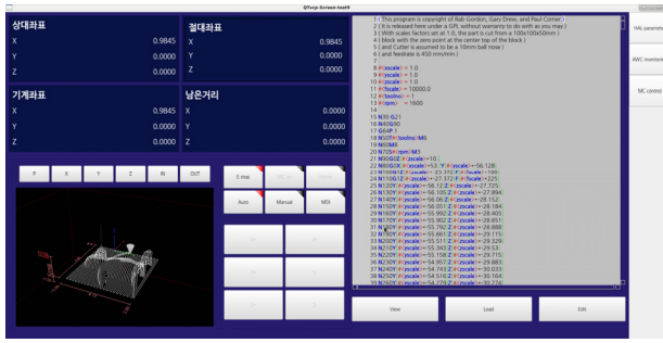
(a) Basic controls: emergency stop, machine on, homing, jog mode, NC loading
