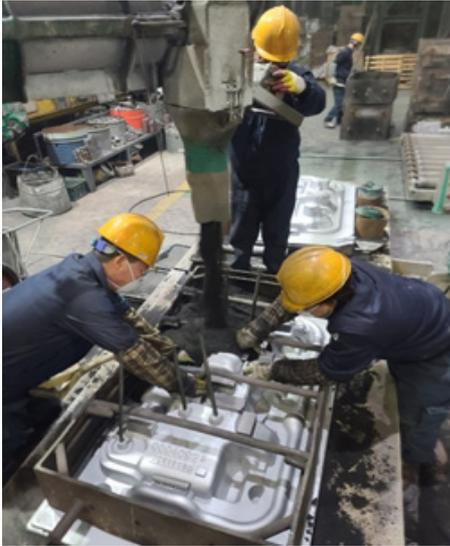
Fig. 11 Molding operation for caterpillar track shoe mold of type 3
