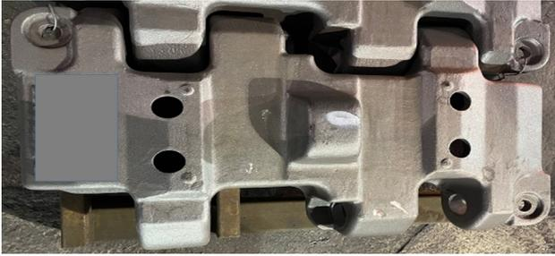
Fig. 16 Caterpillar track shoe parts of type 3 for super-large excavator
