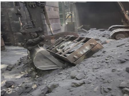
Fig. 13 Sand removal work for caterpillar track shoe mold of type 3
