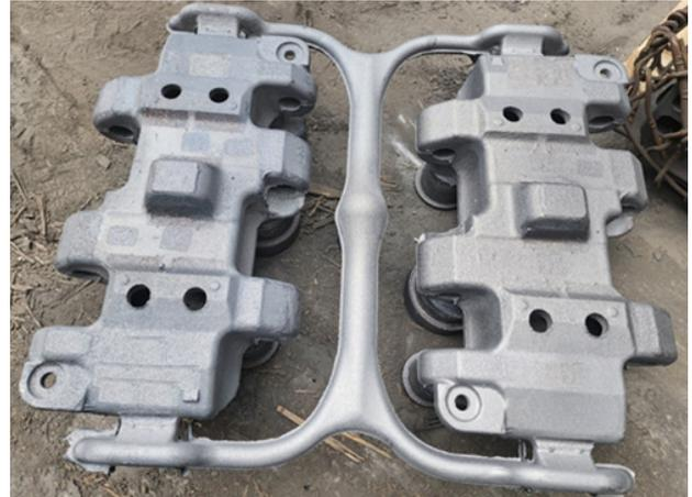
Fig. 14 2 cavity casting process product of track shoe parts after removing sand of type 3
