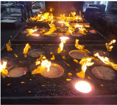
Fig. 12 Pouring operation for caterpillar track shoe mold of type 3
