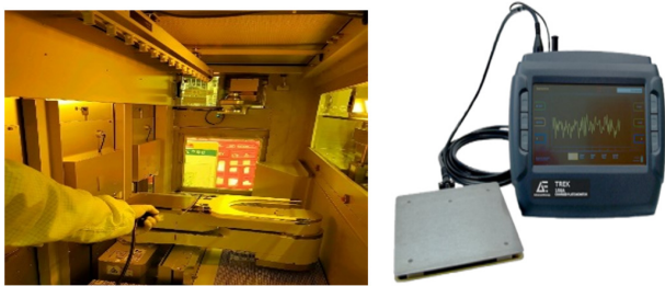
Fig. 5 Status of static elimination performance evaluation in EFEM using CPM
