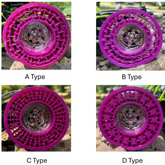
Fig. 9 3D-printed airless tires
