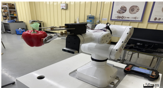
Fig. 15 Example of paprika gripping
