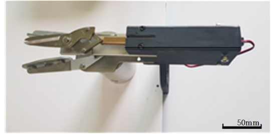
Fig. 11 The grip part and the cutting part are assembled by the robot connector
