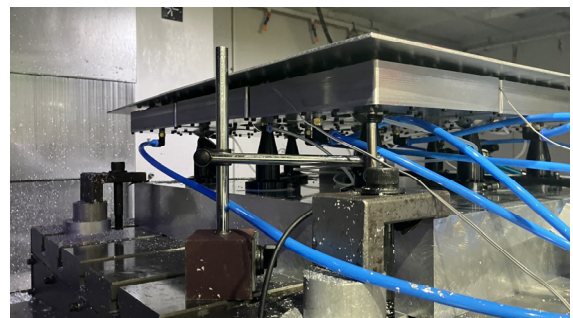
(c) LVDT sensor under fixture
