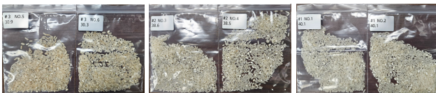
(a) Grinder passed rice (b) Inverter position No. 900 (c) Inverter position No. 800
