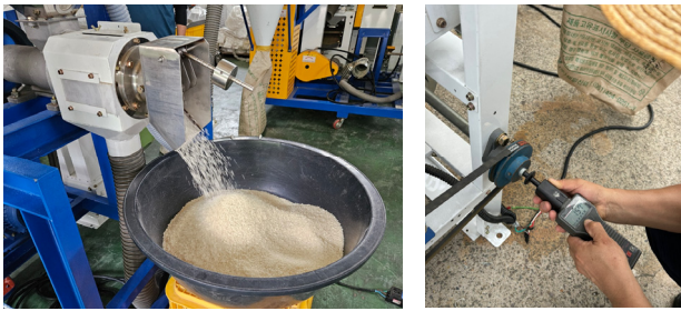
(a) Final production of white rice (b) Measurement of revolution of main motor
