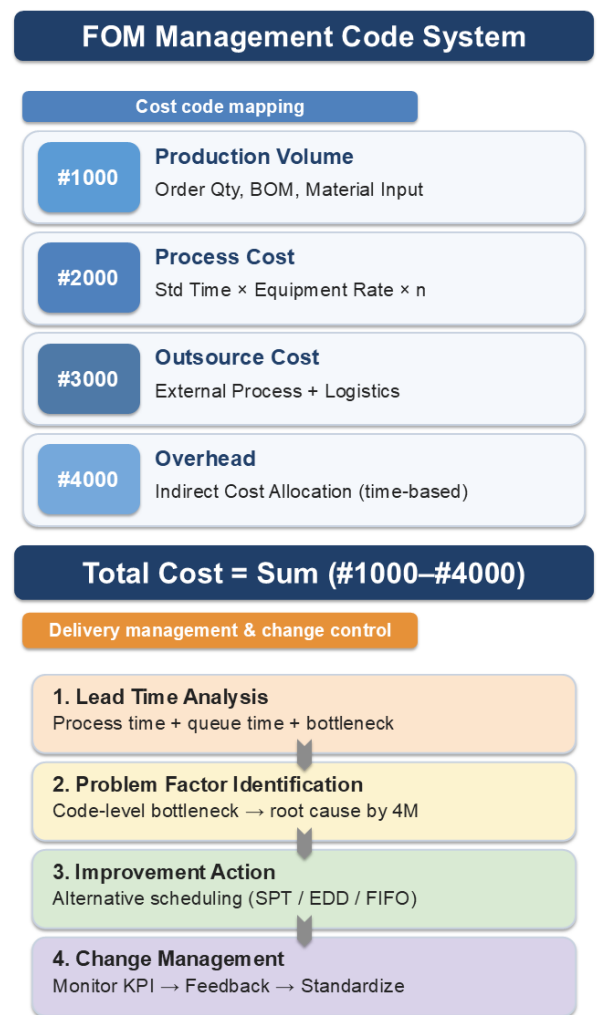
Fig. 3 FOM management code system and delivery change management process
