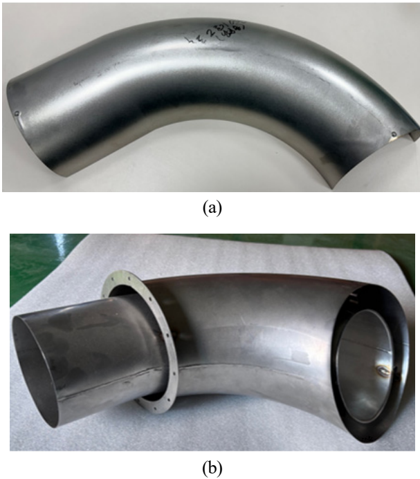
Fig. 10 Final product after (a) trimmed inner part of APU duct and (b) welded APU duct assembly
