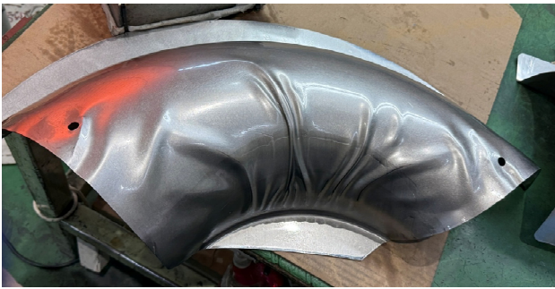
Fig. 5 Wrinkle defect observed in the first forming trial
