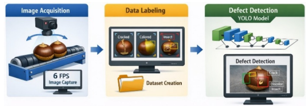
Fig. 2 Overall system architecture for chestnut defect detection
