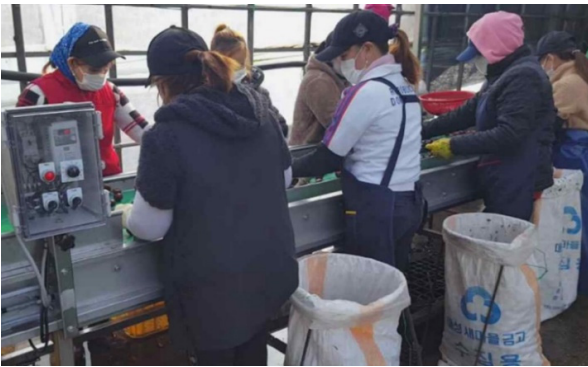
Fig. 1 Manual visual inspection process for chestnut sorting
