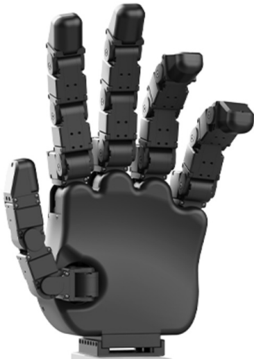
Fig. 3 Examples of robotic hands with 4-revolute-joint thumbs (robot hand of ROBOTIS HX5-D20) [8]
