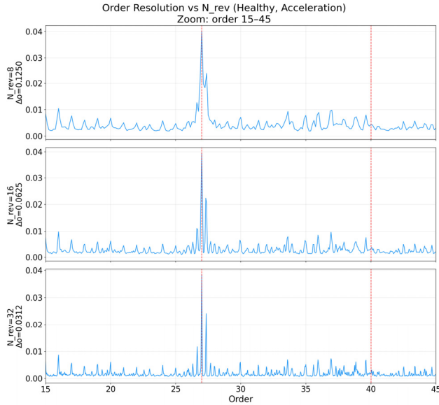
Fig. 3 Effect of window length N_{rev} on order resolution. This figure compares N_{rev} = 16 with 8 and 32 revolutions around orders 15–45 and supports the choice of N_{rev} = 16
