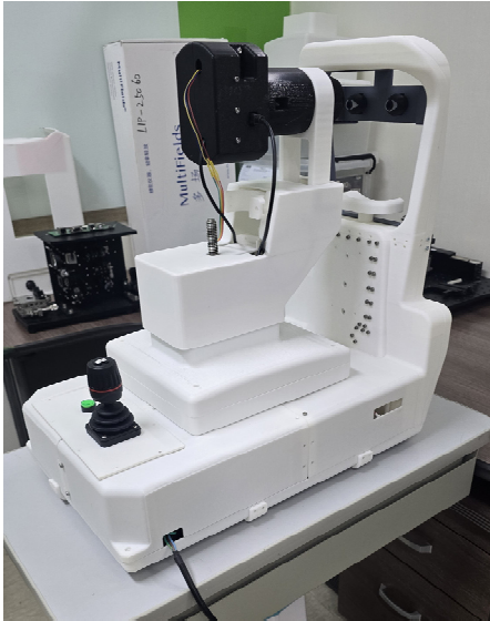
Fig. 8 Experimental setup for automated fundus image acquisition
