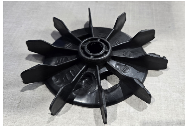
Fig. 1 Deformed impeller part
